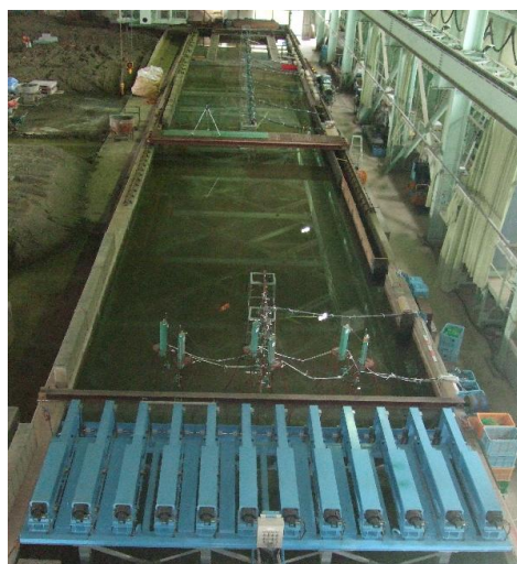
Fig.1 Water tank for wave generating experiments
